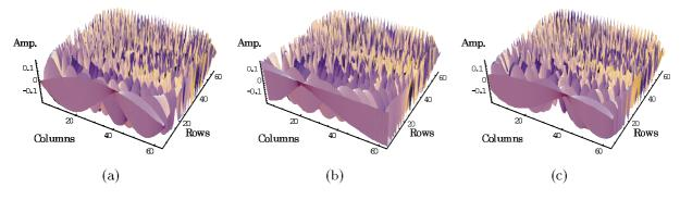
Fig. 2. Modal-wavelet matrices ( $64 \times 64$ ). (a) Dirichlet type boundary condition. (b) Neumann type boundary condition. (c) Green function type.
