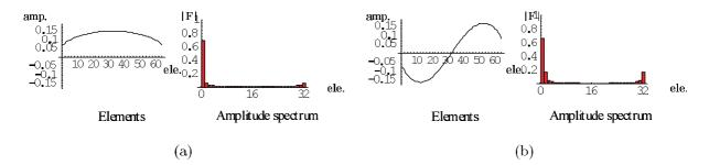
Fig. 5. Elements of row vectors in the matrix shown in Fig. 2(c) and their Fourier amplitude spectrum. (a) The first row vector. (b) The second row vector.
