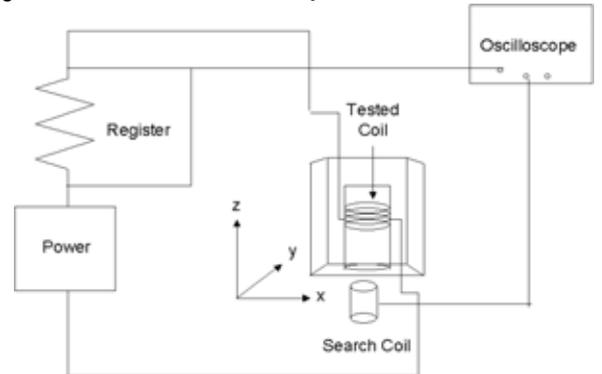
Fig.7 Schematic Diagram of Experiment
