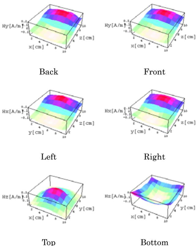
Fig.8 Magnetic Field Distributions at each of the Different Measured Planes
