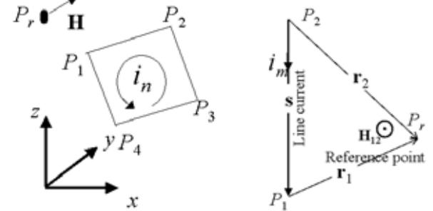
Fig. 2 Rectangular Loop Current Element. Left: Four Line Currents Representing Rectangular Loop Current. Right: Calculation of Magnetic Field Caused by the Line Current from  $P_2$  to  $P_1$
